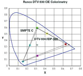
The Runco DTV-930 RGB color triangle almost completely overlaps the SMPTE triangle so nearly all colors in the video signal can be reproduced. The blue and green primary colors are close to the SMPTE standard phosphors and the red primary is shifted to the right. The resulting color accuracy is
